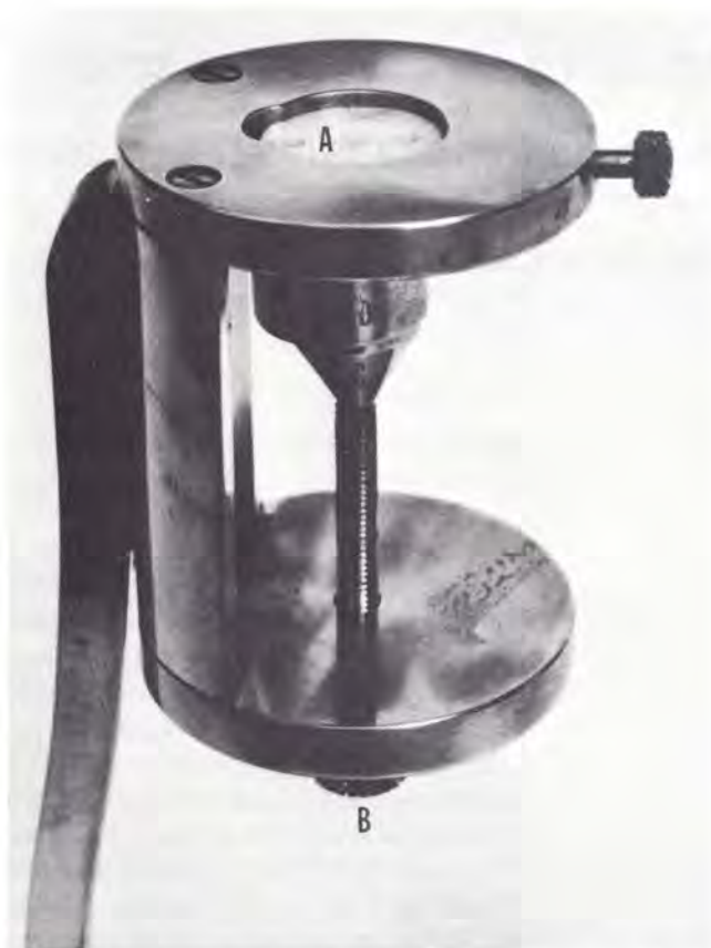
Fig. 1. Initial apparatus for the assembly of test specimens. A) Split teflon mold; B) Knob which was rotated to elevate and lower the elevating platform; C) Platform; D) Tooth embedded in brass tooth cup.
